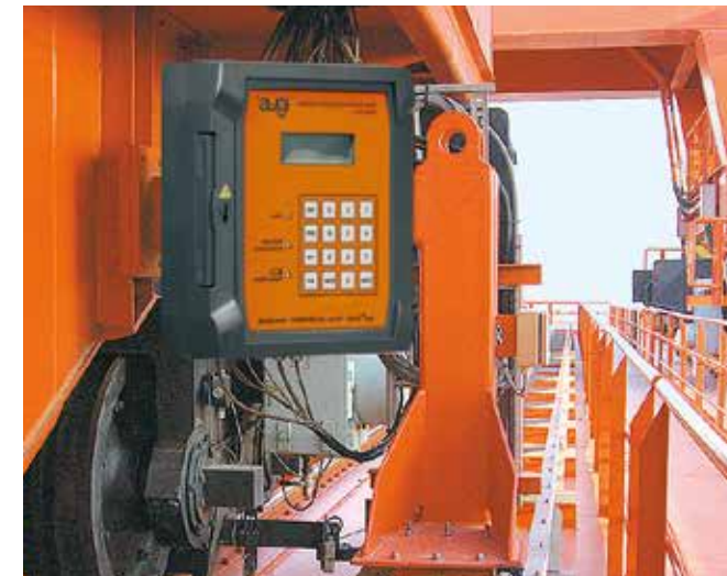
Long travels with electronic push/pull force monitoring with igus® i.Sense EC.P
