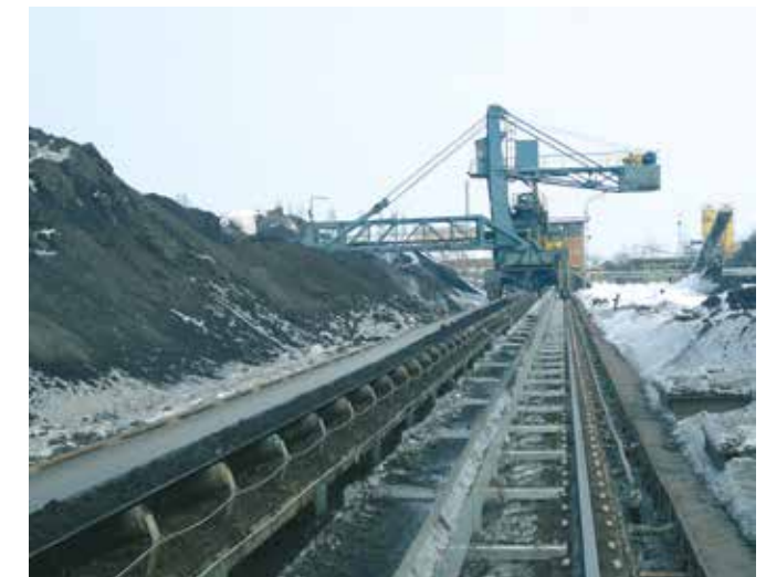
Series 4040HD on 180m travel lengths with housing. Temperature range from -40°C/+40°C and in very dirty environments
